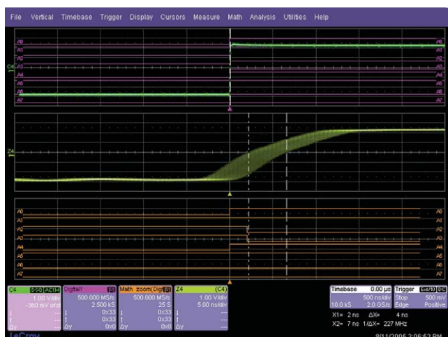
Figure 6. Sample-based pattern triggering generates 4 ns of trigger jitter (LeCroy WaveRunner with MSO option).
