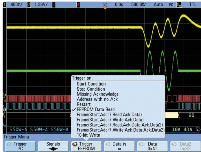
Figure 12. Triggering on a 3-cycle chirp with I 2 C triggering and decode in an Agilent MSO.
