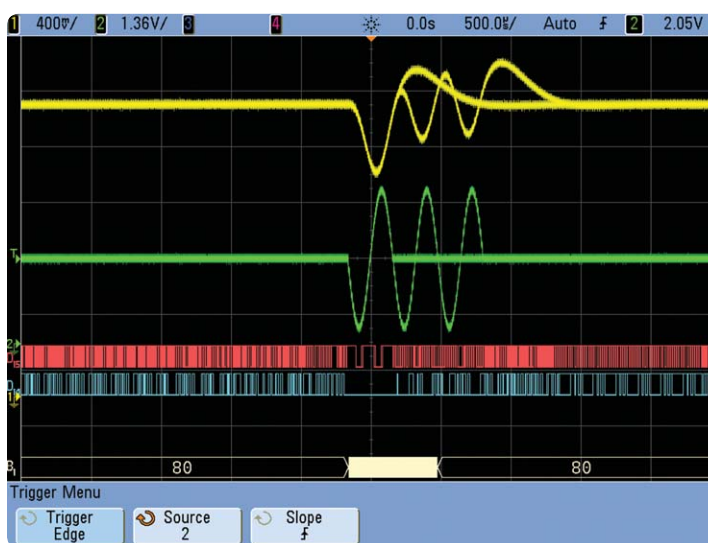
Figure 11. Conventional oscilloscope edge triggering fails to synchronize on specific-length chirps.
