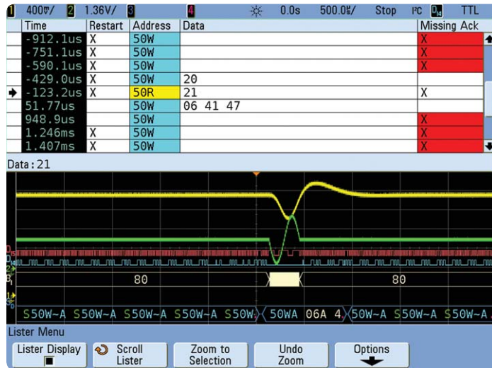
Figure 13. Triggering on a 1-cycle chirp with I 2 C triggering and decode in an Agilent MSO.
